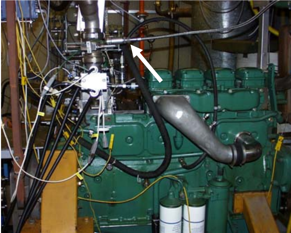
Figure 3. The modified Volvo TD100 engine viewed from the inlet side. The operating cylinder is to the left in the picture.
