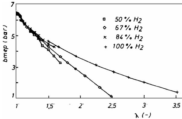
Fig. 9. The bmep for high hydrogen concentrations
