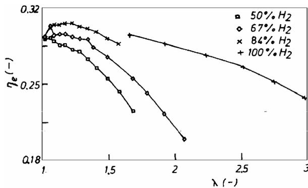
Fig. 10. The efficiency for high hydrogen concentrations
