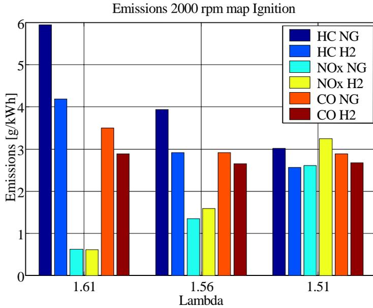
*Emission values from tests with 8% Hydrogen mix into the CNG compared with pure CNG for different air/fuel ratios*
