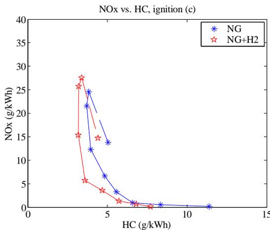
**Figur 7: HC - NO<sub>x</sub> trade-off with natural gas and Hythane. The markers represent different air/fuel ratios. Intermediate ignition timing strategy.**
