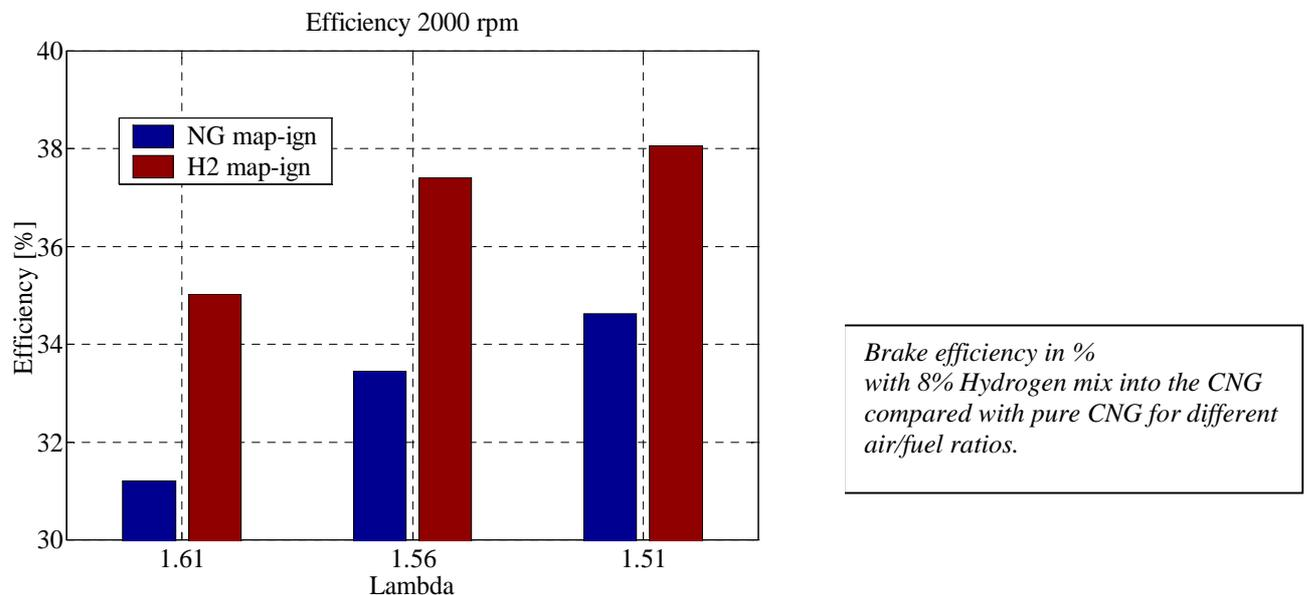
**Fig 4. Brake efficiency 8<sub>vol</sub> % Hydrogen**
